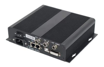
The SVB200 is a standard model of Starview controllers, Undertakes encoding and data processing, sending the audio and video to the LED display. It communicates with PC via USB port for convenience. The SVB200 feature following advantages, better satisfying users' requirements:
